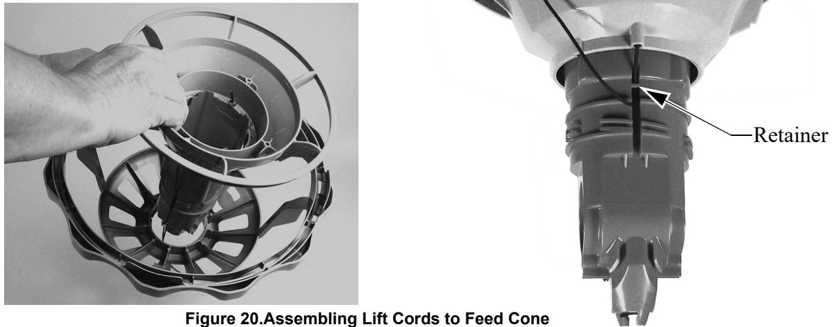
Figure 20. Assembling Lift Cords to Feed Cone
