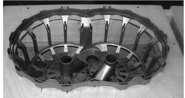
Figure 21. Place Grill into Assembly Fixture
