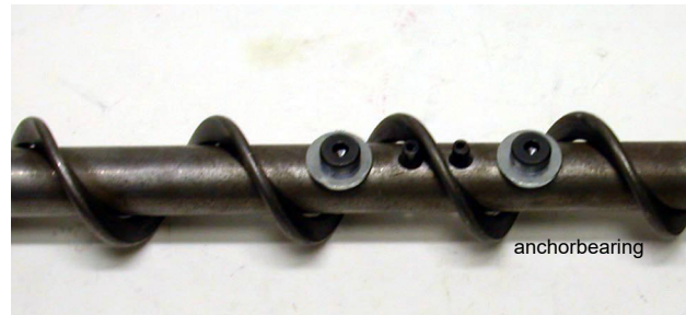
Figure 63. Auger and Anchor Bearing Connection
