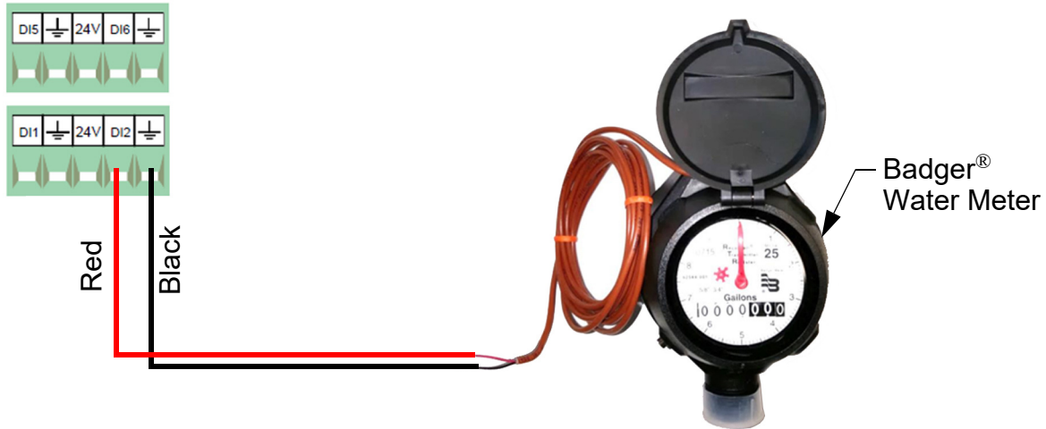
Figure 28. Water Meter Wiring
