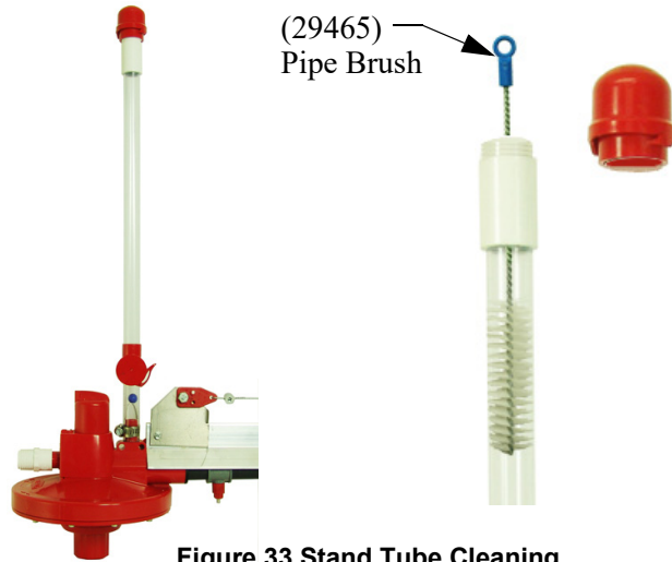
Figure 33. Stand Tube Cleaning
