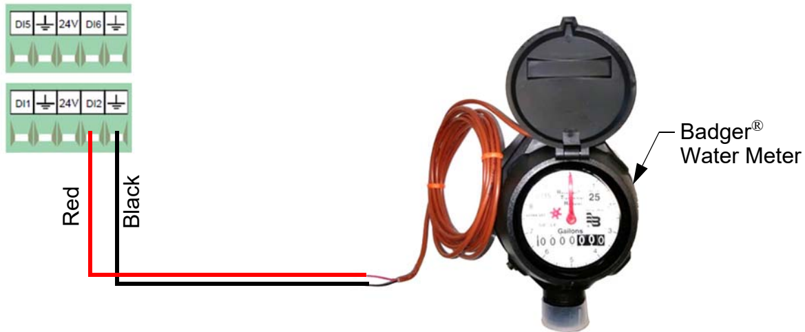
Figure 22. Water Meter Wiring
