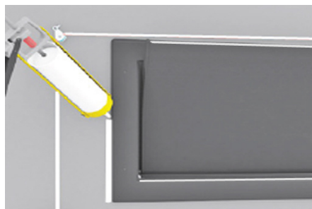
Step 8. Caulk all four sides of Inlet after installation for improved Inlet Performance
