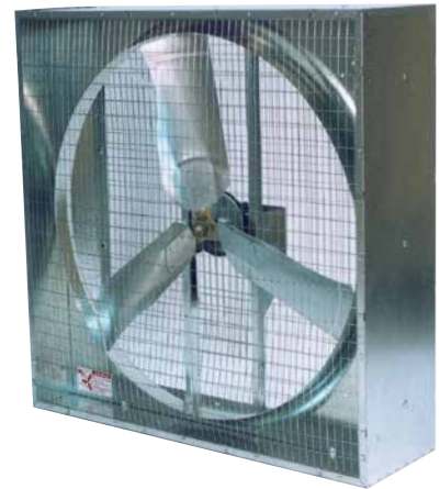
Chore-Time's 91-cm Direct-Drive Box Fans deliver 18,650 m 3 /h and 27.9 m 3 /h/Watt at 0.00 static pressure.
